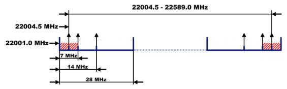
Figure 1.6. Frequency range of the HYPERCABLE CFIP-23 FODU
