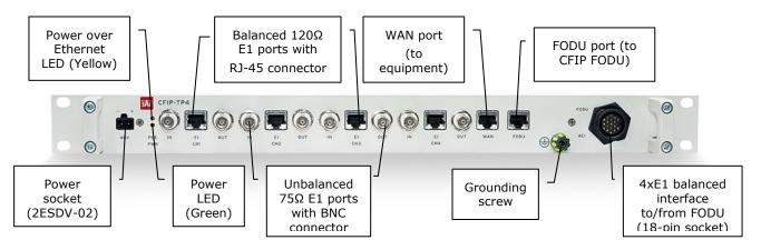
*Figure 2.9.* Termination panel for the HYPERCABLE CFIP FODU; the E1 port numbers on the front panel correspond to the HYPERCABLE CFIP FODU port numbering.
