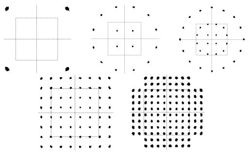
Figure 5.15. Constellation diagrams – QPSK, 16APSK, 32APSK, 64QAM, 128QAM
