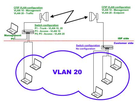
Figure 4.11. VLAN configuration with 'Access' VLAN
