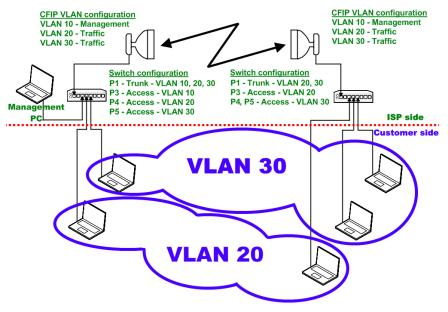
Figure 4.10. VLAN configuration with VLAN tag encapsulation on the ISP side
