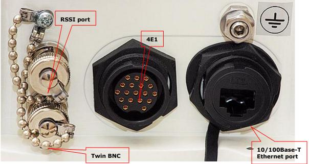
Figure 1.3: Detailed view of HYPERCABLE CFIP FODU connectors
