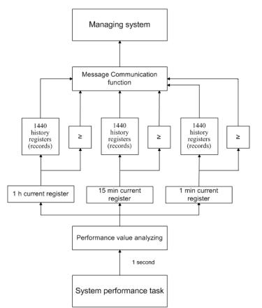
Figure 5.6. Functional architecture for data collection, history and thresholding treatment
