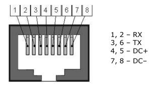
Figure 9.2. RJ-45 socket pin number
