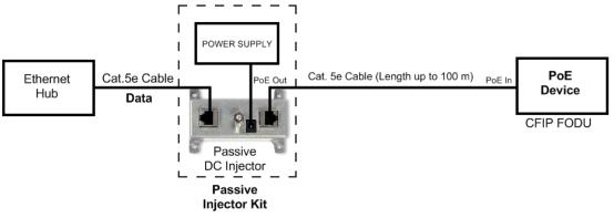
Figure 2.7. Power over Ethernet passive injector application
