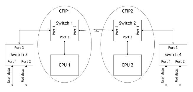
Figure 4.7. System with VLANs
