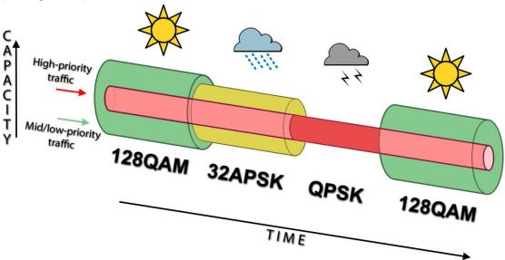
Figure 4.2. ACM bandwidth capacity adaptation
