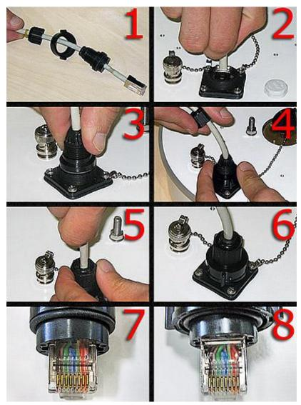
Figure 2.1. Assembling Ethernet weatherproof connector
