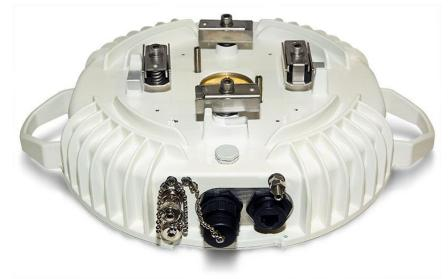
Figure 1.2: HYPERCABLE CFIP FODU connectors
