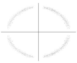
Figure 5.13. Phase noise (QPSK)
