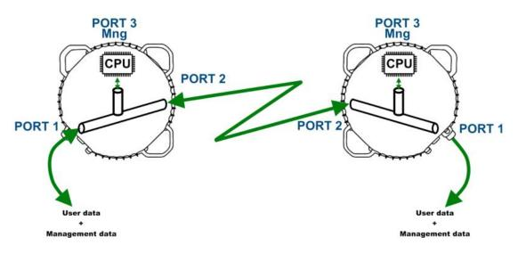
Figure 4.6. System without VLANs
