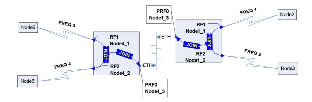
In this example we have joined several distributed (possibly even geographically distributed) network segments (in previous examples we had a similar situation and the solution was in using trunk groups; **join+prf** combination is much more convenient). Combining "joins" for different radio interfaces and pseudo radio interfaces the network will obtain a good number of alternative paths in any direction thus providing with the best delivery quality and less bottlenecks.
