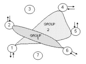
Therefore, MINT network can be viewed as one virtual distributed switch where border nodes act as external ports of the switch. Switch task is to transparently transport packets from one external port to another one (other ones). Important to understand that switching groups should be created only at the nodes where packets come to or from "outside" network ("outside" relative to MINT). On the repeater nodes there is no need to create switching groups regardless the topology.
