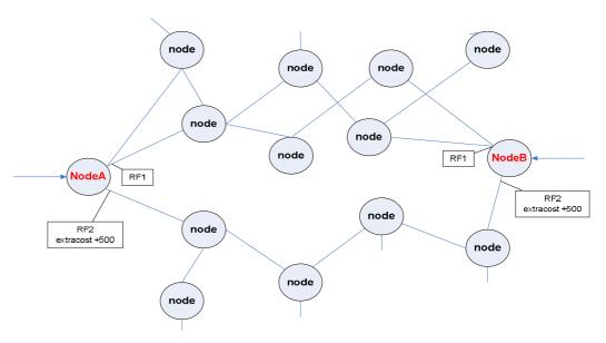
For example, we want the streams between NodeA and NodeB to use upper side of our network segment so that lower part of the segment would be used for inner streams of the segment. This is accomplished by using "**extracost**" parameter as shown on the diagram (the value of **extracost** parameter should be chosen based on other costs on the node).
