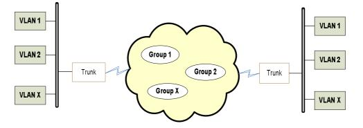
As packets originated by internal MINT network nodes do not belong to any of the switching groups, special command "**switch local-tag N**" is used to send them through the trunk group.
