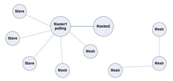
Now, if Master1 turns marker access (polling) on, the network will disintegrate into two separate segments:
